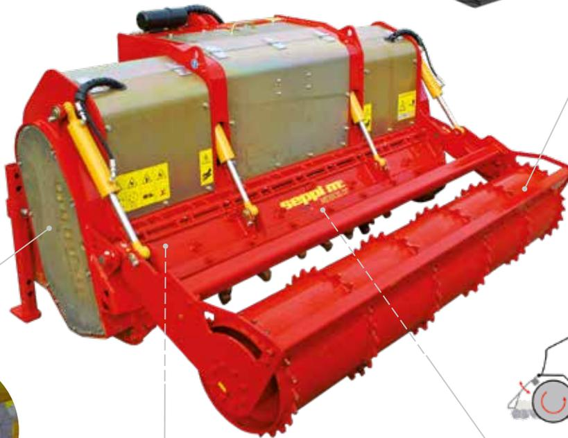
Hydraulically operated compacting roller for depth control, may also be used as guard frame incl. roller scraper (option)
