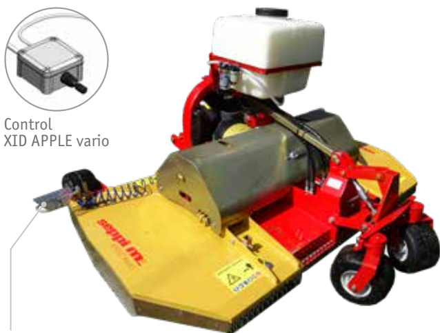
APPLE vario: Adjustable nozzles holder with anti shock - transparent nozzles cover
