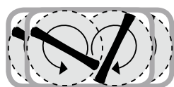
Overlapping blades for a regular cut, also while changing the working width
