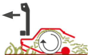
Open rear hood: to mulch grass with low power consumption
