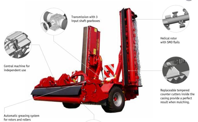
the large diameter improves mulching on uneven ground.
