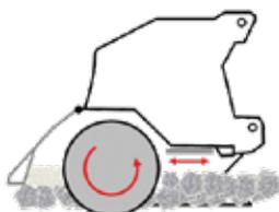
Adjustable anvil bar to adjust the degree of mulching; easy adjustable by screws.
