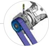
**CARBONCHAIN™** belts provide high strength and length stability with high flexibility
