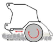
Adjustable anvil bar to adjust the degree of mulching
