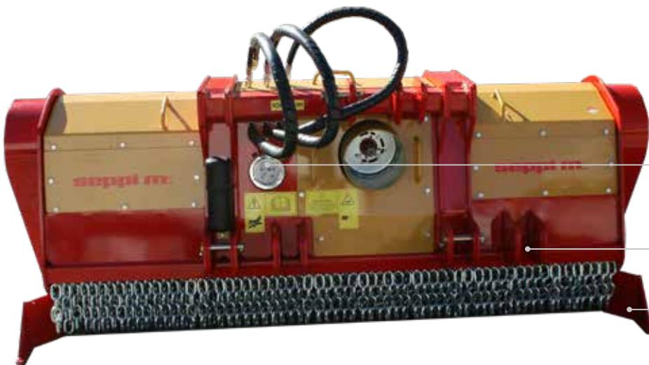
Pressure gauge to control surface pressure of the grader blade
