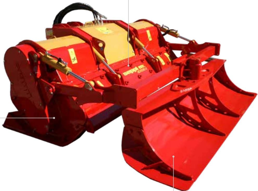
Grader blade (option), hydr. height and rotation adjustment, with hydraulic pneumatic damping incl. lateral extensions
